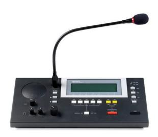
Interpreters can easily select the incoming languages of their choice by using the 5 relay preset buttons with red indicator LED. These buttons are easily programmed by pressing and holding the relay preset button and cycling through the available language channels on the LCD display with the up and down controls. Releasing the relay preset button programs the selected language. The relay preset is activated by pressing the white relay button with green LED indicator.
